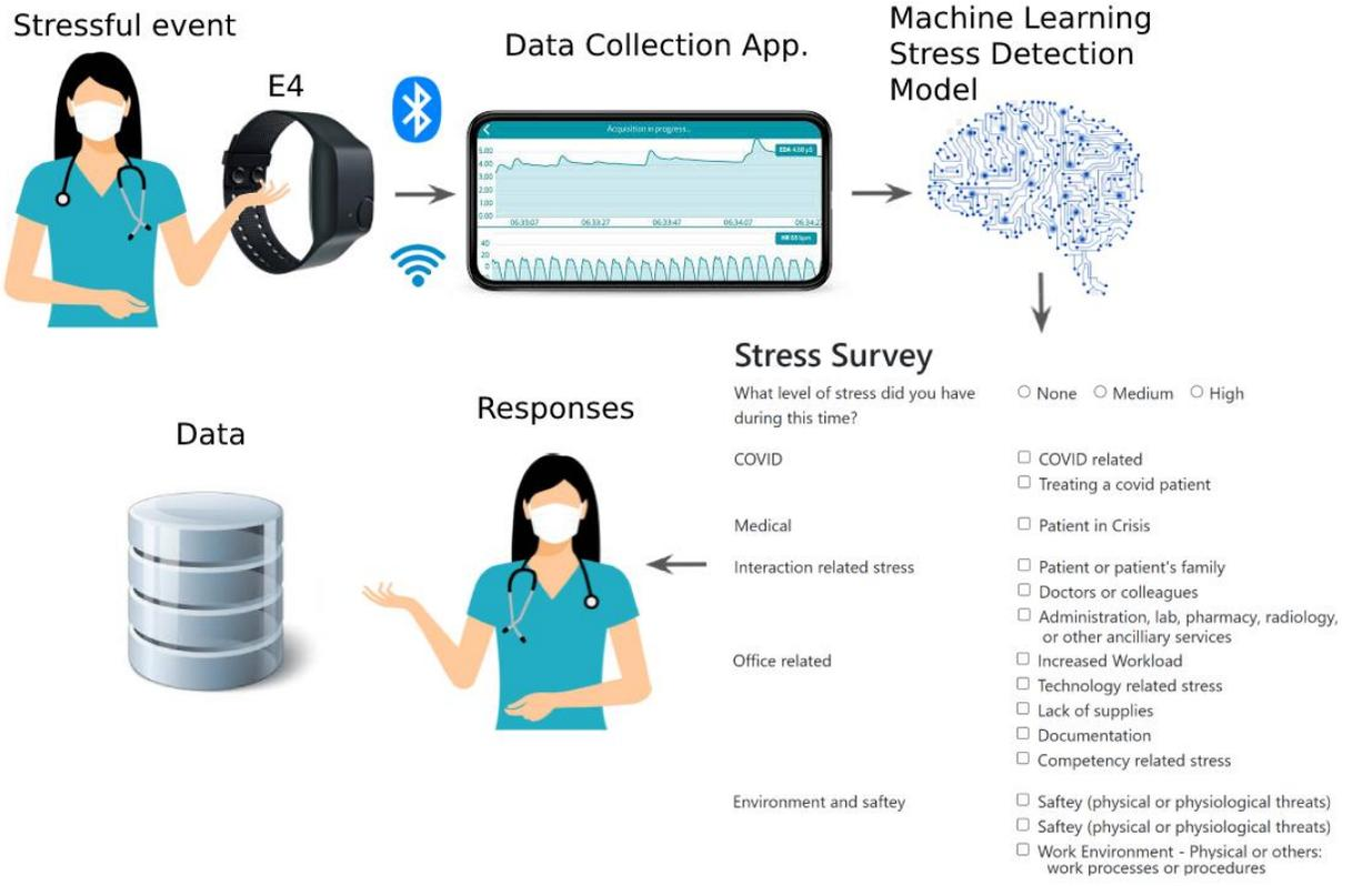
**Figure 1 Description of Stress Detection Apparatus**
